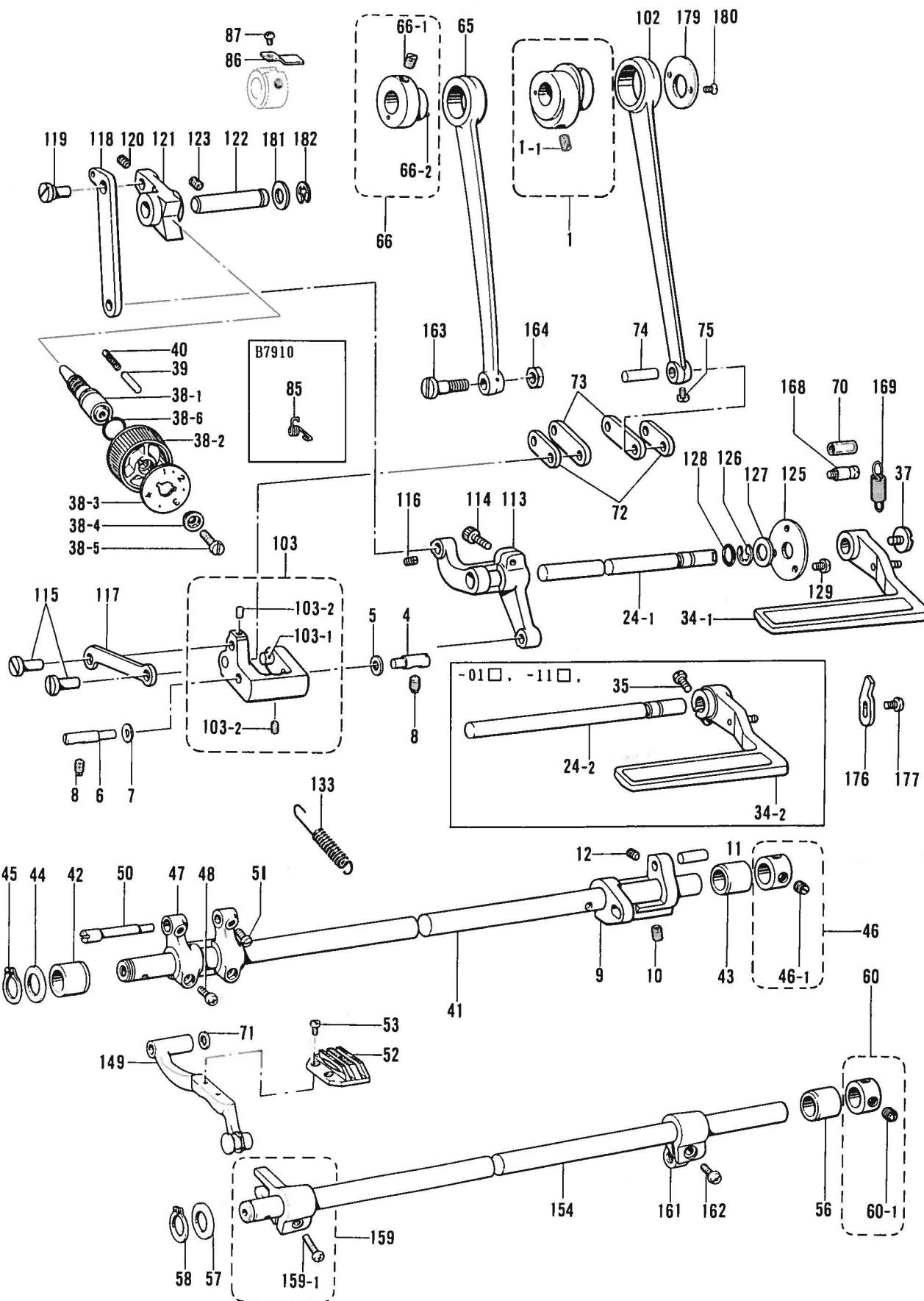
F. 送り関係/Feed mechanism/Transportvorrichtung/
