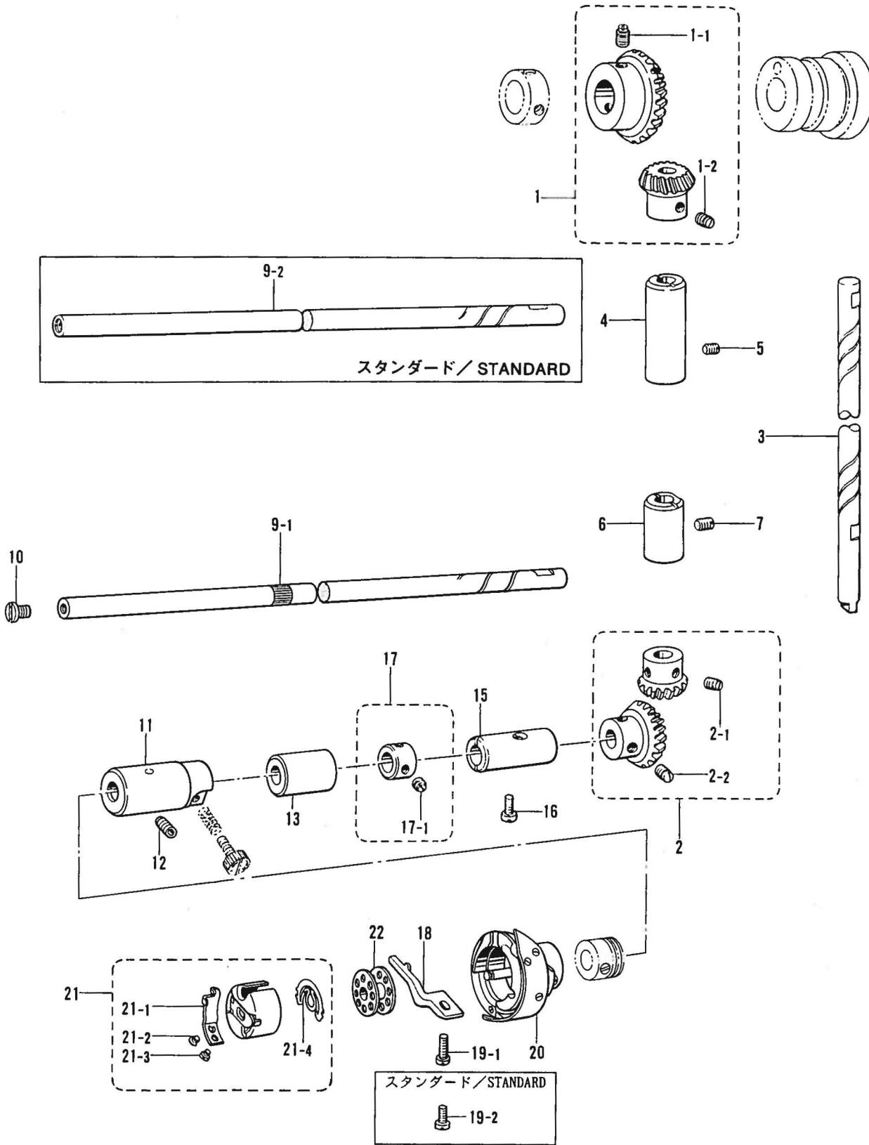
J. カマ関係/Rotary hook mechanism/Greifervorrichtung/
