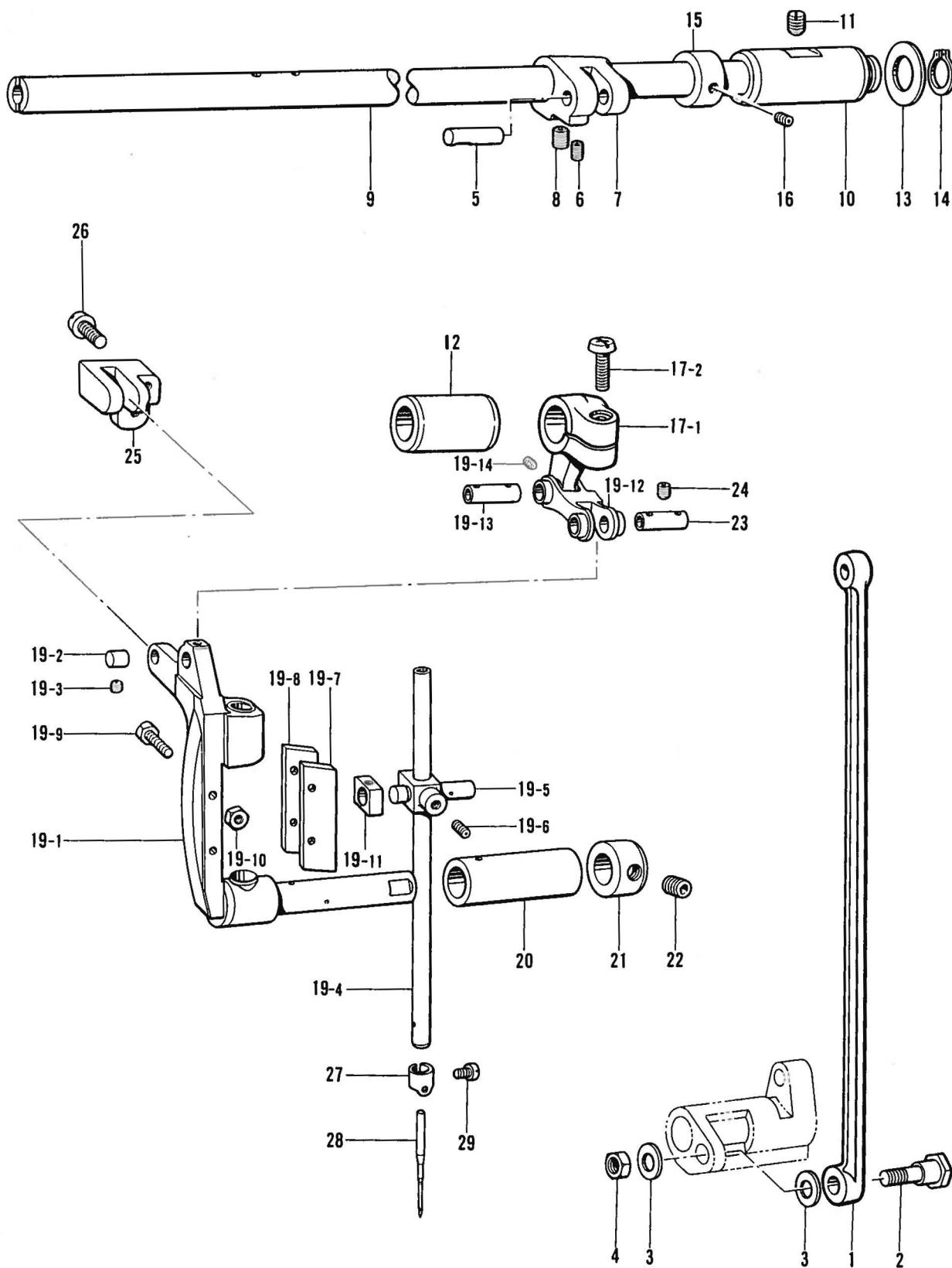
D. 針送り関係/Needle feed mechanism/Nadelstange transportvorrichtung/
